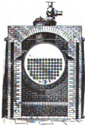
FIG. 20.—SECTION OF TUBULAR BOILER AND SETTING.
